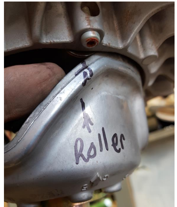
Figure#5. roller position and marks aligned (stock helix before removal shown for reference)
