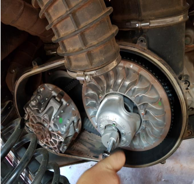
Figure 1- spread secondary(rear) pulley
